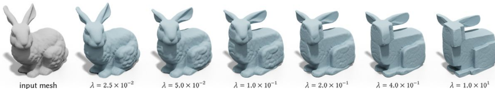
Fig. 9. One can control the CUBENESS by changing the \lambda parameter in Eq. 1.
